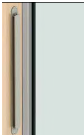
Click vent. Anodized surface finish. Fully concealed. Free ventilation opening in elements with 24mm glazing: 4000mm 2 . Free ventilation opening in elements with 48mm glazing: 3000mm 2 . For the equivalent free opening, please refer to our website.
