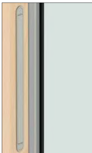
Click vent. Anodized surface finish. Fully concealed. Free ventilation opening in elements with 24mm glazing: 4000mm 2 . Free ventilation opening in elements with 48mm glazing: 3000mm 2 . For the equivalent free opening, please refer to our website.
